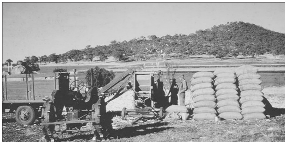
Richter corn sheller in action at "Echo Dell", Saddletop, Clifton. Logan Hoey feeds the cobs onto the elevator while Bruce Hoey watches the bags filling.
