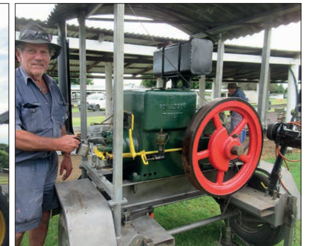
At the Heritage Weekend, Lester Diggles demonstrates his Ronaldson Tippett "CA" Crude Oil Engine. It starts on Kero and runs on sump oil and diesel- there are only 2 in Australia still going. Lester, who now comes from Warwick, grew up on the family property at Glengallan Flats.
