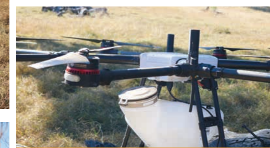
The spreading drone can hold seed, fertiliser or granules of whatever description, making it effective for a variety of uses.
