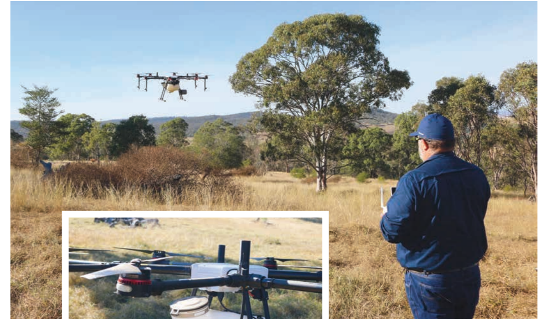
The spreading drone can hold seed, fertiliser or granules of whatever description, making it effective for a variety of uses.
