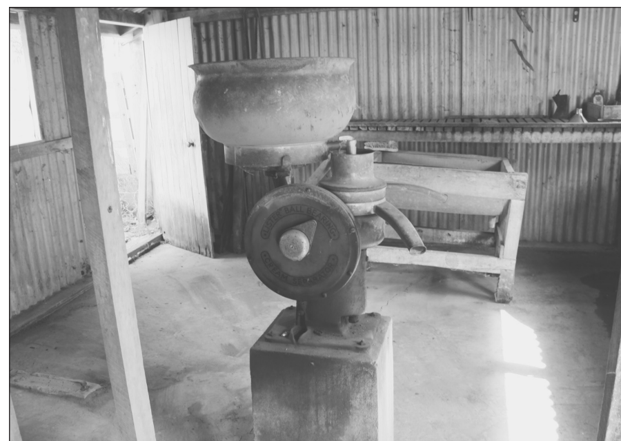
Cream Separator in engine and separator room.
